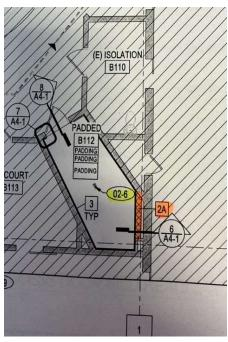
**Answer:** The pop out must have been copied from a past set of drawings. It is no longer in the cell and therefore there is no need to fur out the wall.
